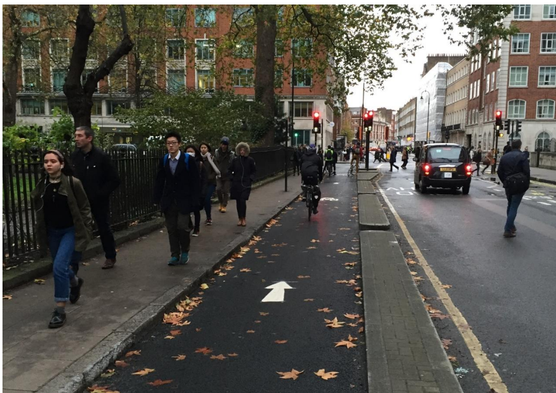
Figure 4.3: With traffic flow - segregated cycle track - Examples
